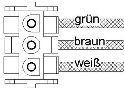
*Im. 2: Terminal diagram connector (top view)*
