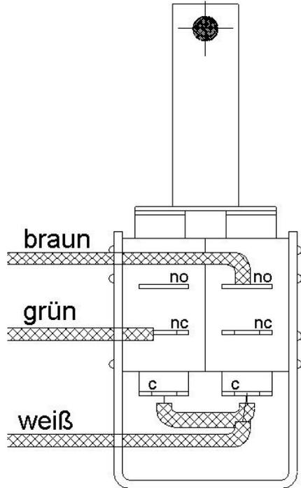
Im. 1: Terminal diagram door contact switch
